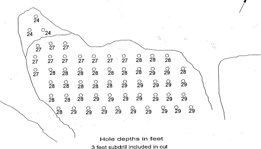
3 feet subdrill included in cut Approximately 56 Holes Drill Pattern 9 feet x 9 feet Hole diameter 4 inches
